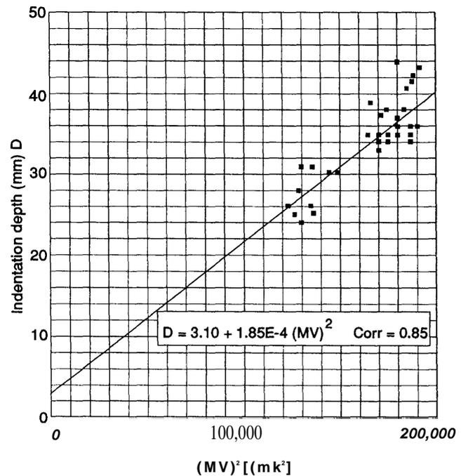
NOTE: Mark 22 9-mm bullets fired from a Thompson Contender with a 10-inch Barrel at Panels of 20-ply, 1,000denier, Kevlar-29 on Roma Plastilina No. 1 Modeling Clay Conditioned in Accordance with NIJ Standard 0101.08.
